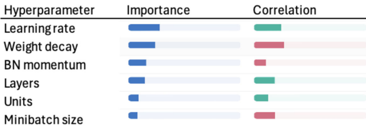
Fig. 6 Estimated feature importance metric for each hyperparameter, and linear correlation between each hyperparameter and the validation loss. A green correlation bar indicates a positive correlation and a red correlation bar indicates a negative correlation
